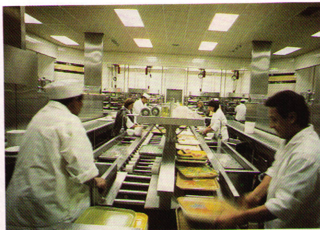
Duncan Hall's tray accumulator system affords employees a quick and efficient method of cleaning up between meals. Trays are funneled via conveyors to a central area for easy scraping and dishwashing.
